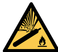
Warning against pressurized cylinders
